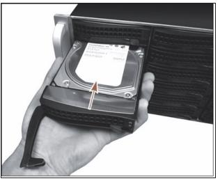
**Figure 320** Install the drive into the BlackPearl gateway.
