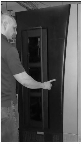
**Figure 245** Press the door release button to open the door.
